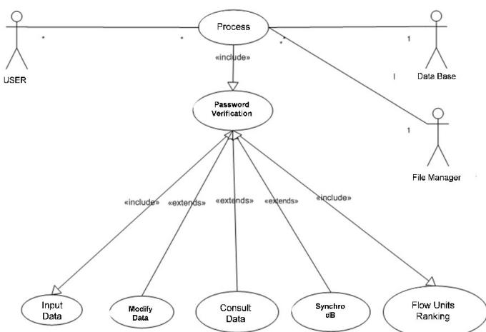
**Figure 14.** User Initialization & Software Process for “SFP”.
