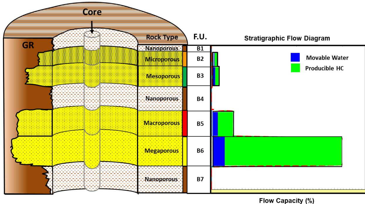
**Figure 20. Characterized fining-upward geological sequence showing Stratigraphic Flow Diagram. 100% Flow Capacity of units highlighting “producible fluids” type. Movable Fluids (Water + Hydrocarbon) Flow Unit.**
