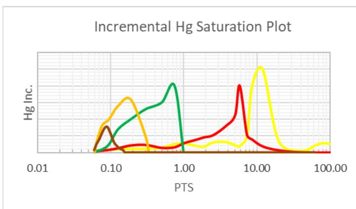
**Figure 11. Incremental Saturation curves derived from High Pressure Mercury Injection tests vs Pore Throat Size selected from available Core Samples & classified by rock type. These curves correspond to the previously selected Relative Permeability samples (Laboratory Data). (B6-Megaporous “yellow”, B5-Macroporous “red”, B3-Mesoporous “green”, B2-Microporous “orange” and B1-Nanoporous “brown”).**
