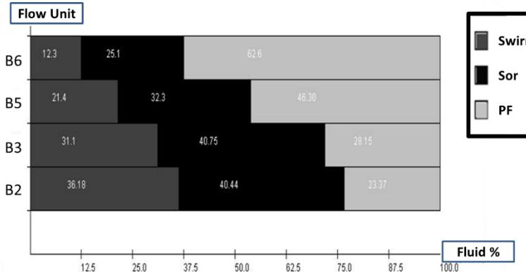
**Figure 13.** Flow Unit Ranking according to “Producible Fluids” (PF).
