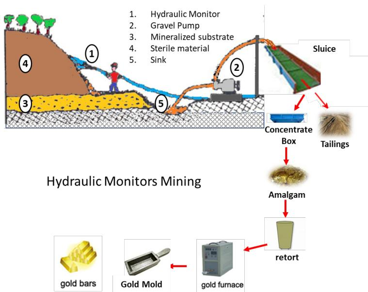
**Figure 2. Hydraulic Monitors Surface Mining.** (Modified from Quaglia & Barbettia, 1991).
