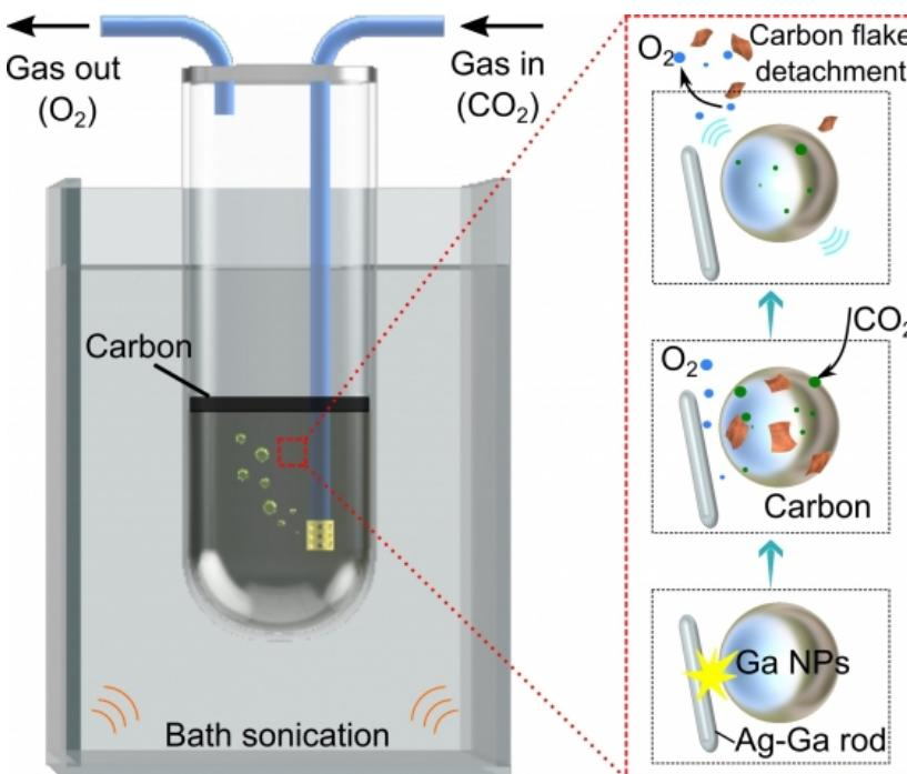
UNSW researchers have helped show how carbon dioxide can be broken down cheaply and efficiently via a process that dissolves captured CO<sub>2</sub> gas into a solvent around nanoparticles of gallium.
