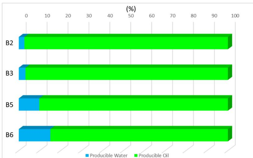
**Figure 17. Flow Units Ranking according to Theoretical Oil-water ratio.**
