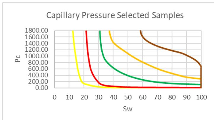
**Figure 10.** High Pressure Mercury Injection Capillary Pressure vs Pseudo Water Saturation curves selected from available Core Samples & classified by rock type. These curves correspond to the representative samples by Rock Type (Laboratory Data). (B6-Megaporous "yellow"; B5-Macroporous "red"; B3-Mesoporous "green"; B2-Microporous "orange" and B1-Nanoporous "brown").
