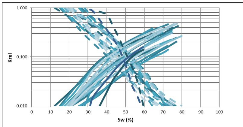
**Figure 8. Krw and Kro curves from selected Core Samples. (Laboratory Data).**
