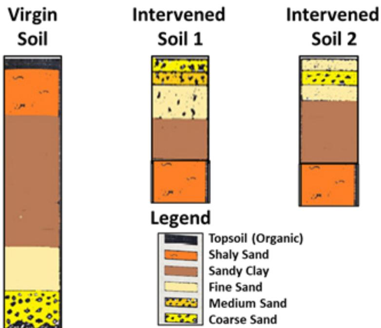
**Figure 9.** Comparison of profiles of both virgin and intervened soils where the granulometric “inversion” is observed in the attempt to recover the soils as a consequence of the colluvial and alluvial gold mining activity. Study Area. It is obvious how the clay layers in the intervened areas are shallower, which would generate a much sooner saturation of infiltration waters than it would naturally, producing eventual floods with its consequences. (Quaglia & Barbetta, 1991).
