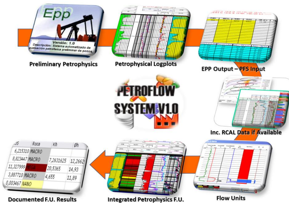
**Figure 5. PetroFlow System (PFS) Workflow for Flow Unit Identification.**
