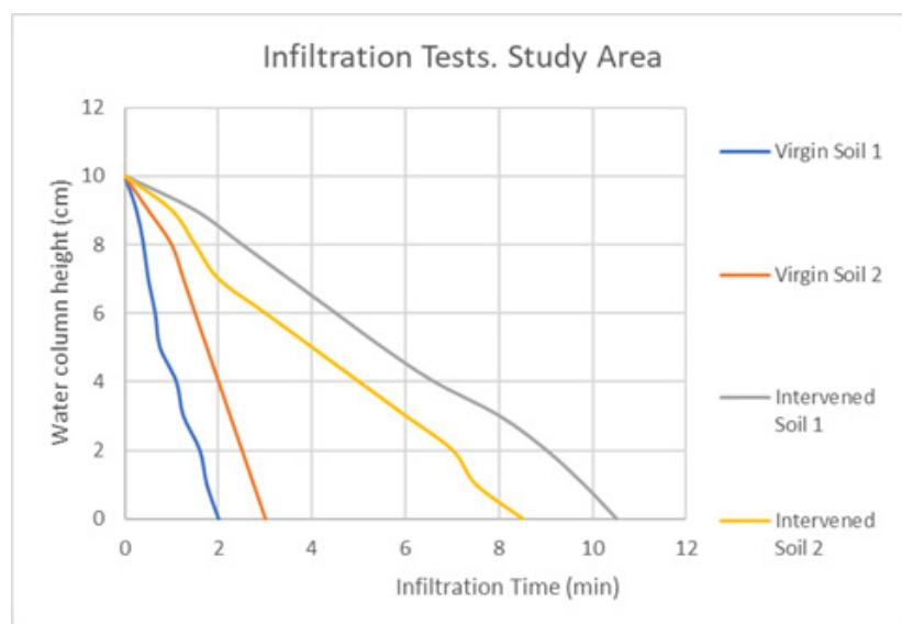
**Figure 10. Infiltration tests on virgin and intervened soils. Study area.**
