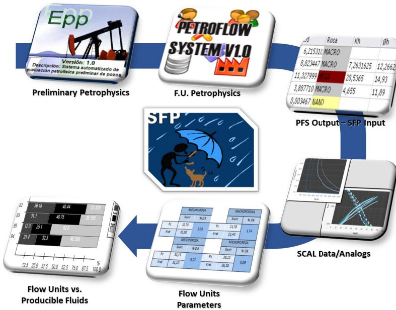
**Figure 7. Productive Fluids Saturation (SFP) Workflow. Flow Units Ranking based on Rock Quality and Producible Fluids.**
