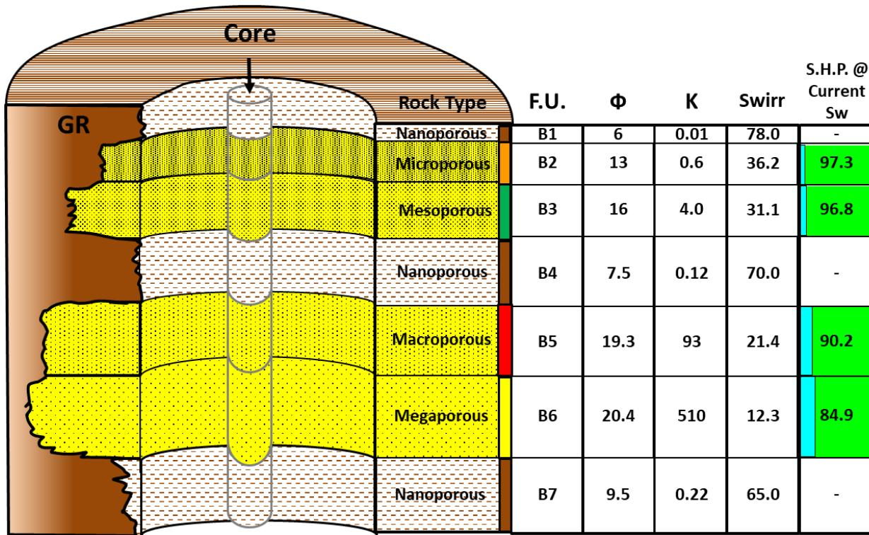
Figure 18. Characterized Fining Upward Sequence with Flow Units Numerical Analysis. Last Column Highlights Movable Fluids with “Producible Hydrocarbon Saturation” values.
