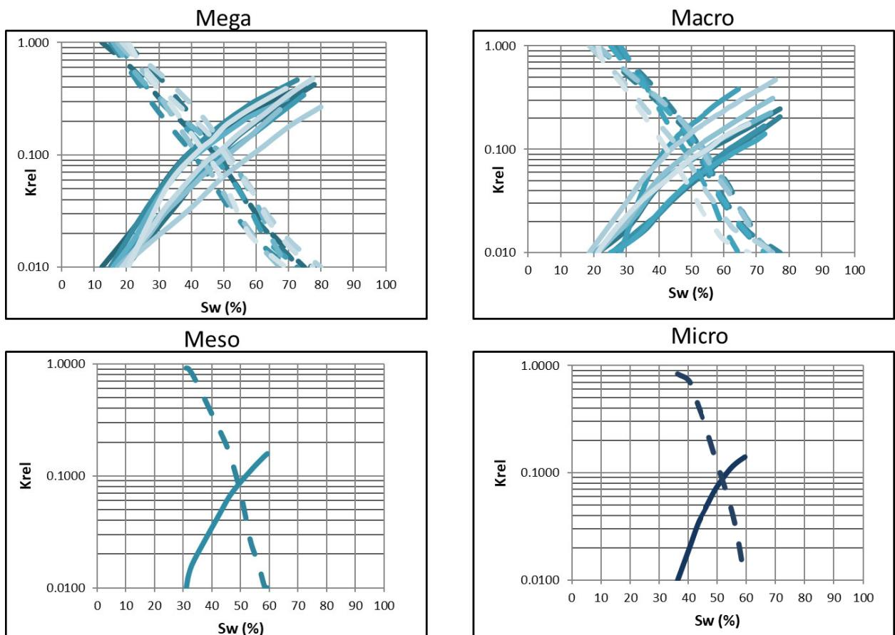
**Figure 9.** Oil-Water relative permeability curves set from selected Core Samples & classified by rock type. (Laboratory Data). (Megaporous, macroporous, mesoporous and microporous).
