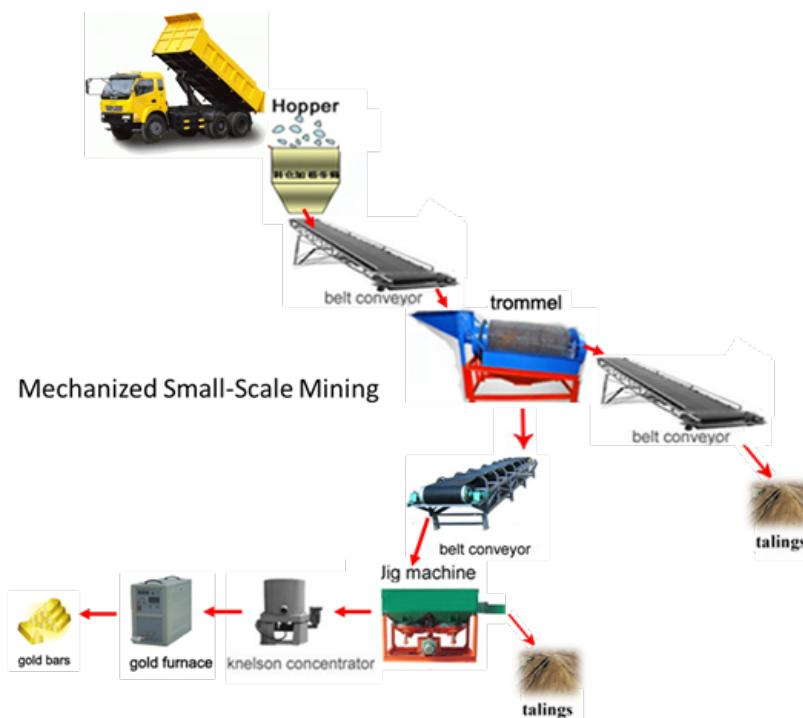
Figure 4. Small-Scale mechanized mining method workflow.
