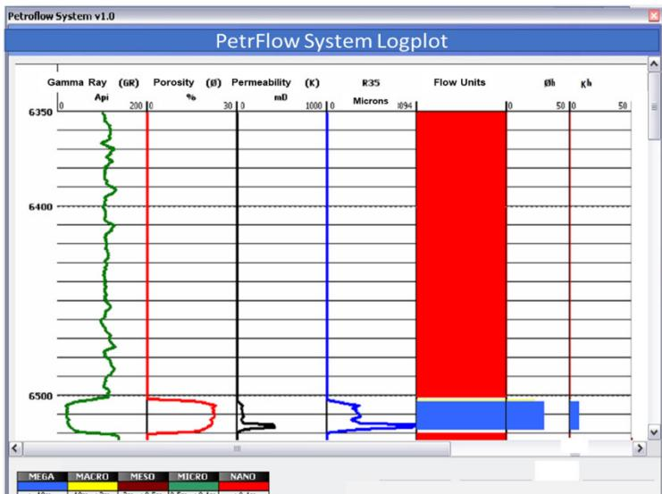
**Figure 6. Automated Flow Unit Identification by detecting Pore throat size contrasts using PFS.**
