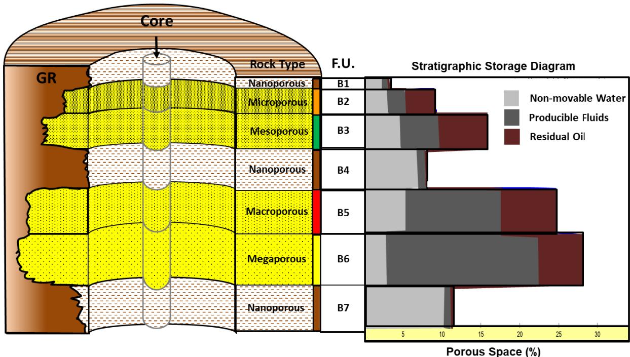
**Figure 19. Characterized fining-upward geological sequence showing Storage capacity of flow units highlighting the mobility characteristics of the fluids contained in them: non-movable water, mobile fluids and residual hydrocarbon.**
